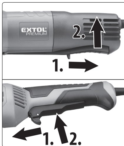
Fig.15; step 1. unlocking, step 2. starting
